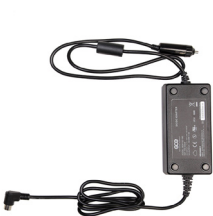
DC (12v) power supply unit
