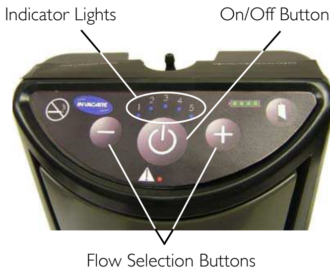
FIGURE 6.9 Adjusting the Pulse Flow Setting
